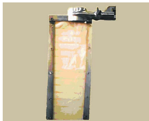
Fig. 1 Mostashari's flammability tester with a treated fabric inserted and pinned in its internal splits, before to the fulfillment of the flammability test
